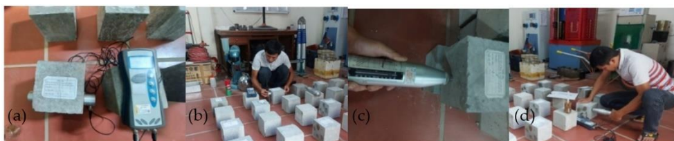
Fig. 1. Experiment to determine concrete compressive strength by an ultrasonic pulse machine Matest - C369N (a, b) and rebound hammer Matest - C380 (c, d) of Italy
