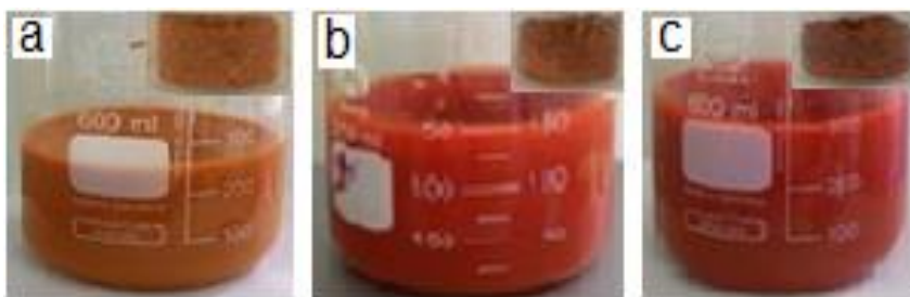
Fig. 2. Colour of Cu 2 O in reaction mixture and in powder state with different NaOH concentrations: 0.5 M (a), 1.0 M (b), and 1.5 M (c)
