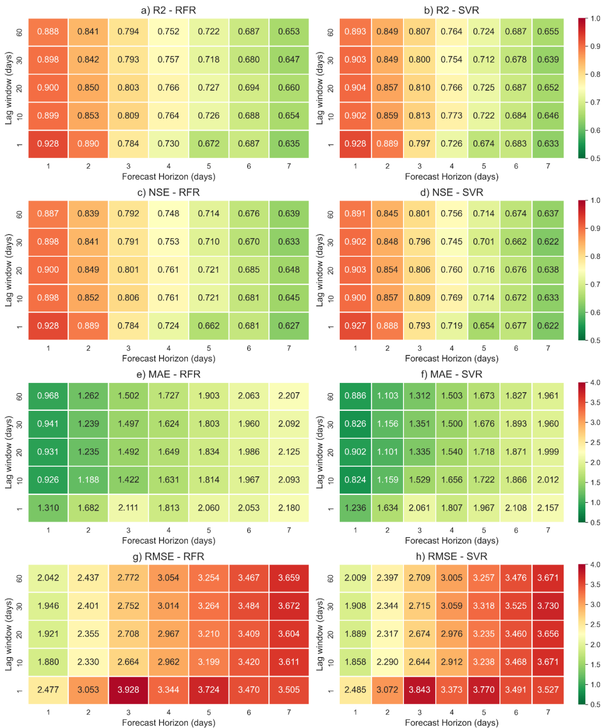
Fig. 4. Performance heatmaps of RFR and SVR models across different lag windows and forecast horizons. Each cell represents the performance score for a specific combination of a lag window (y-axis) and a forecast horizon (x-axis). The color intensity corresponds to the metric value, with higher R^2/NSE and lower MAE/RMSE indicating better model performance.
