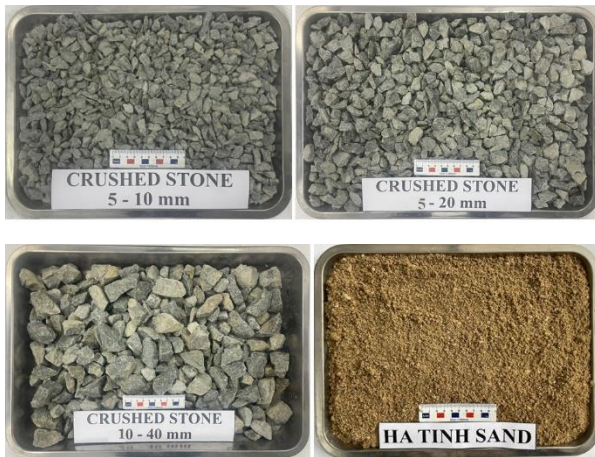
Fig. 5. Photos of crushed stone and Ha Tinh sand samples
