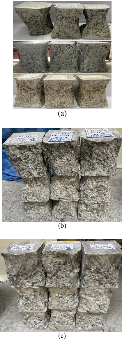
Fig. 7. Photos of SS concrete specimens after compression test: (a) BC510; (b) BC520; (c) BC1040. For each concrete type, specimens from bottom to top correspond to water-cured ages of 3, 7, and 28 days
